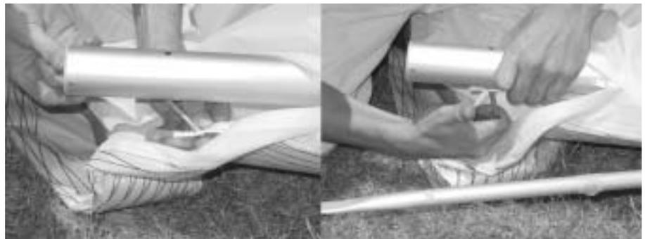
5. Repeat 1-4 to install the left back section. Your Litesport will now be ready for standard assembly. Before each flight, carefully inspect all tubing, nuts, and bolts, to ensure no damage has occurred during transportation.
