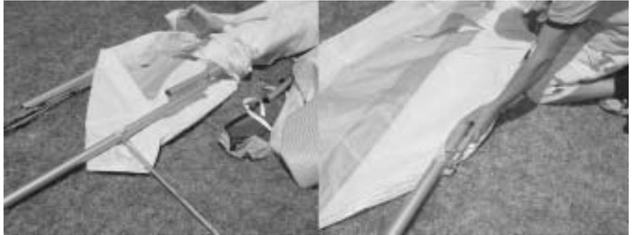
4. Secure the sail by attaching the tip webbing to the end of the leading edge, using the clevis pin and safety ring supplied. Insert the pin through the webbing and into the bottom hole at an angle. Straighten the clevis pin while sliding the webbing towards the leading edge as shown in Picture 3. Ensure the tip webbing is not twisted and is on the bottom of the leading edge.
