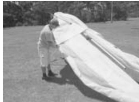
13. Attach the sail ties loosely around glider, going from the wing tip to nose. Then tighten the ties, moving from nose to wing tip. Adjust the sail such that the leading edge Mylar inserts overlap smoothly with no kinks, as shown.
