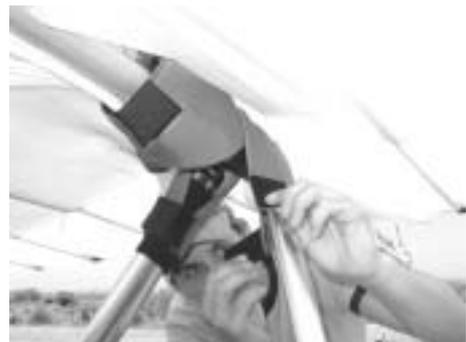
5. De-tension and remove the fibreglass tip.
