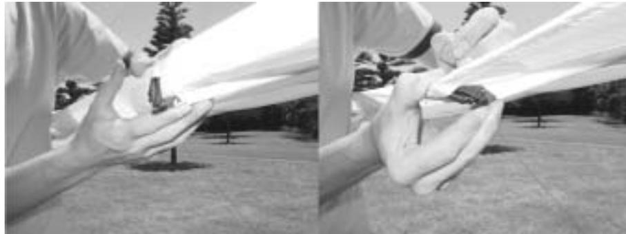
15. Secure the outer wire braced dive strut by rotating it into the sail below the webbing loop. The action of closing the cord wise zipper creates the loop necessary to hold the strut in place.
