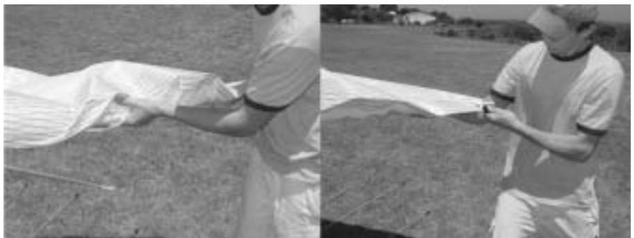
12. Fit the aluminium cup of the tip lever to the end of the tip rod and tension tip by rotating the flat end of the tip lever inboard. For extra leverage, place your thumb through the loop that is attached to the end of the tip lever. Make sure the tip lever is locked against the tip rod. Close the zipper.
